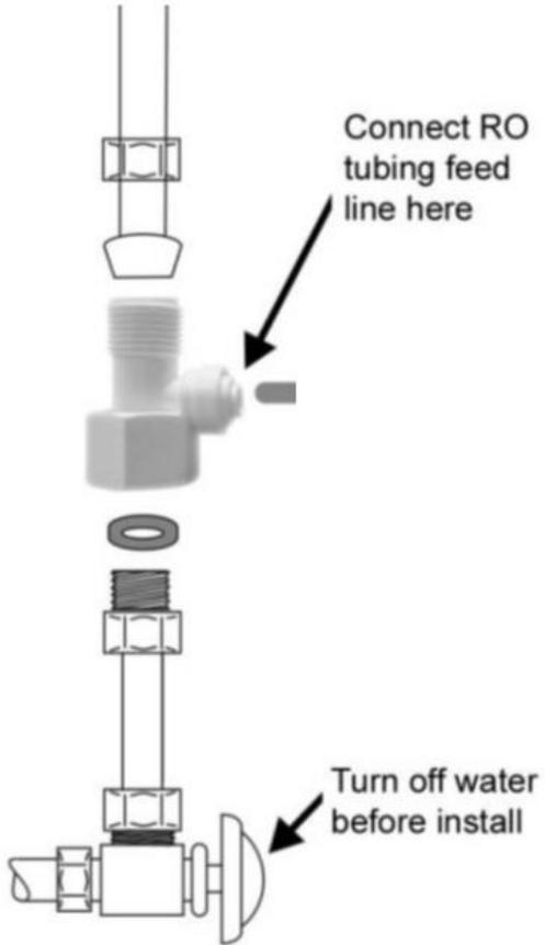
Feed Water Valve Installation
