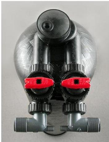
View from the top. Unit with bypass installed. The elbows can point any way that's convenient for the installer. Water enters this filter from the right side. The picture shows the unit in bypass position.
